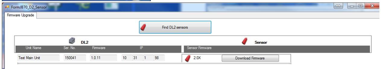
Older sensors may show 2.0X, this is because they are not programmed to respond. New softwares in new sensors will respond with the software version (2.13, 2.14 etc.). If in this older case, ensure the sensor is connected and that values are currently being received from the sensor.
